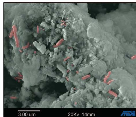
*E-SEM Photomicrograph showing likely IRB rods at MIC corrosion site*
