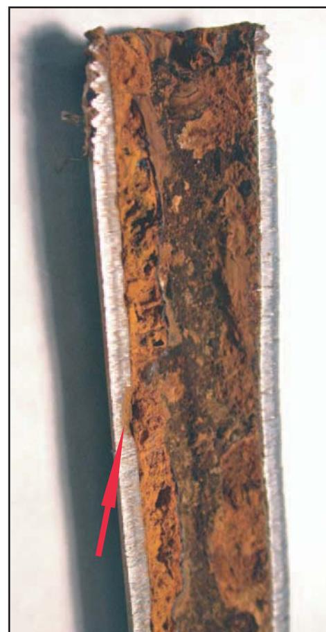
*Cross-section of galvanized pipe showing MIC effects. Note: pitting has reduced wall thickness by 60%.*
