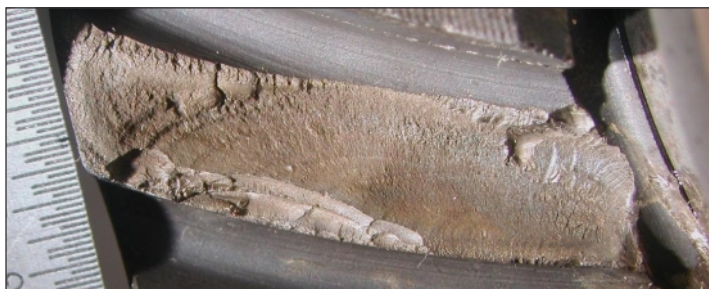
Gear tooth fracture, showing beachmark features characteristic of high cycle fatigue.
