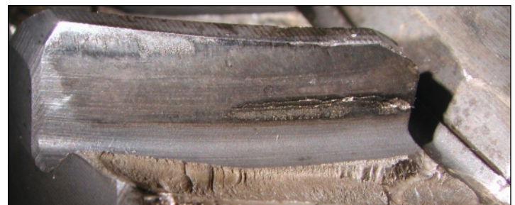
Secondary gear tooth damage consistent with long-term wear.
