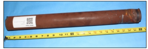
Submitted boiler tube exhibiting corrosion.
