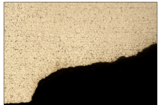
Tube microstructure at corroded area.
