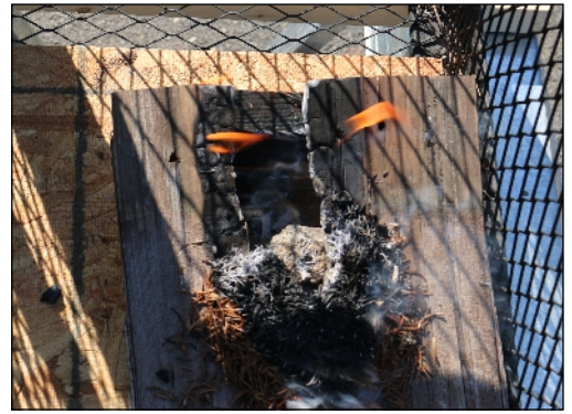
Controlled testing of debris to shingle.
